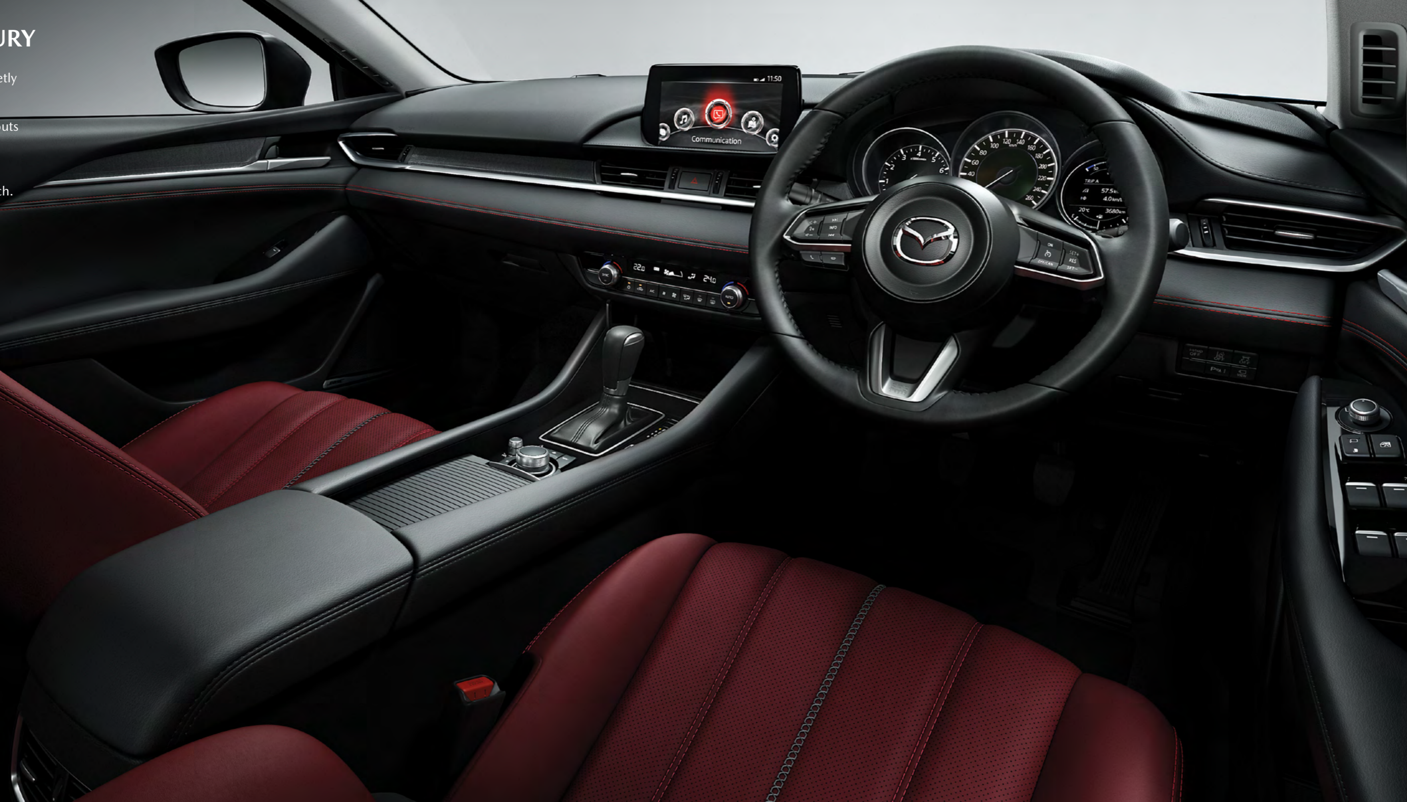
Mazda Connect 8-inch TFT LCD multi-information touchscreen display now features 360° View Monitor. (2.5L & 2.2L Diesel Variants Only)
